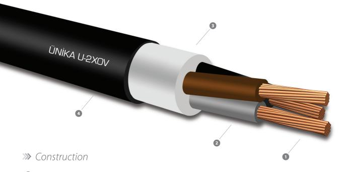
1 Conductor : Bare stranded or compact copper in accordance with IEC 60228 Class 2 Insulation : Cross-linked polyethylene, XLPE in accordance with IEC 60502-1
